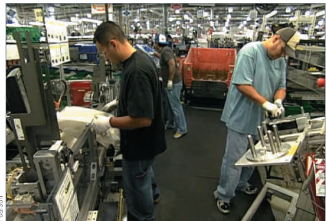
Autoliv employee folds an air bag in a Toyota-inspired production cell.
